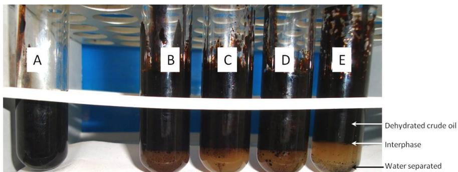
**Figure 8.** Photographs showing separated water (WS) from the initial O/W emulsion containing GlyC<sub>12</sub> (1000 ppm) at 50 W, 60°C. Initial O/W emulsion before MW irradiation (A), emulsion after MW irradiation during 2 (B), 4 (C), 8 (D), 10 minutes (E).
