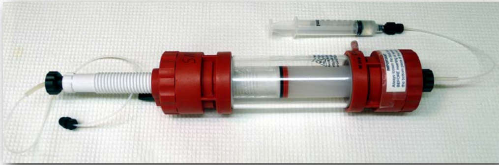
Figure 8.3 -- An ion exchange column apparatus
