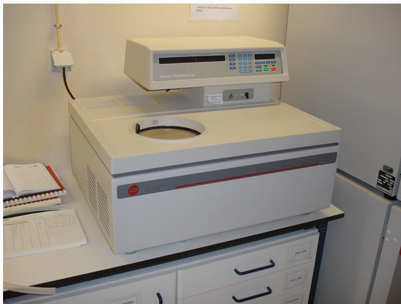
Figure 8.2 - A high-speed centrifuge can be used to obtain different cell fractions from a crude lysate
